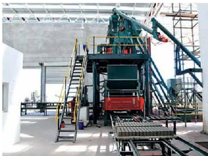
A VB4X machine from PMSA with a capacity of up to 110 000 bricks per nine-hour production shift
