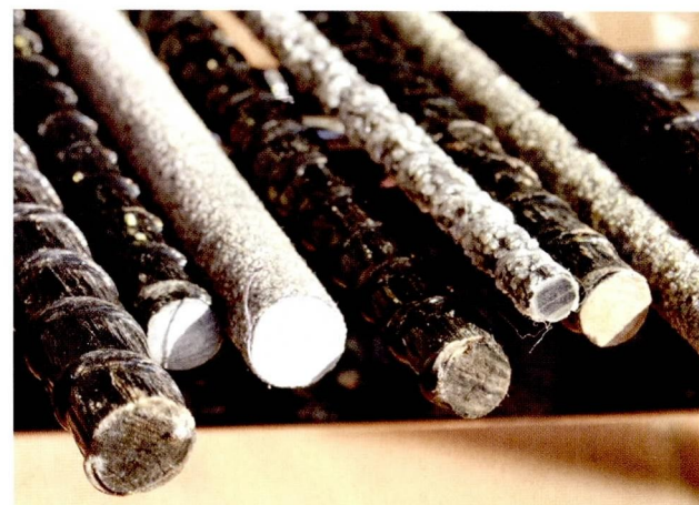
Basalt Technology’s StoneRod rebar offers a cost-effective and corrosion-proof alternative to conventional steel or glass fibre reinforcing.
