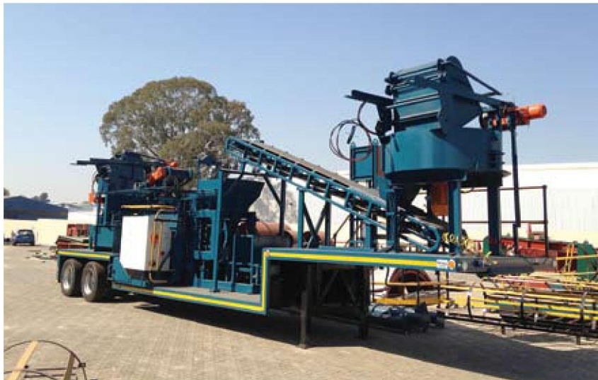
The trailer mounted RE600 mobile block machine, designed and manufactured by Pan Mixers, is capable of producing 20 000 high quality paving bricks per shift
