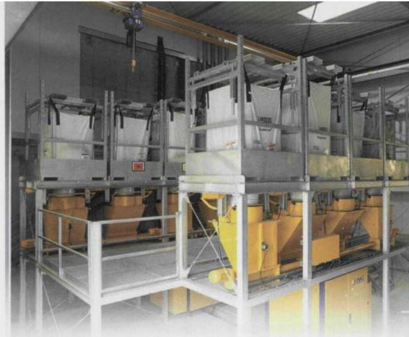
The Finke universal powder pigment dosing system
